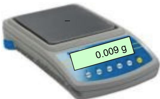
Figure 3. Electronic balance shows one significant digit in a measurement
