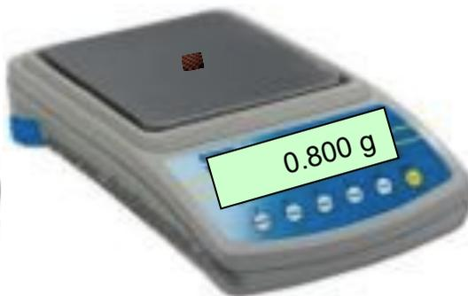
Figure 2. Electronic balance shows three significant digits in a measurement
